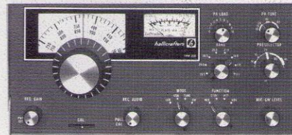
Control Panel of FPM-300, done in handsome grey and black, consists of Main Tuning Control; Receiver Audio; Mode (LSB/USB/CW/Tune); Receiver Audio; Calibrator Adjust; PA Load; PA Tune; Mic/CW Level; Preselector; Function (Receive/Standby/PTT/VOX) plus Plate MA panel meter and large frequency readout display.
