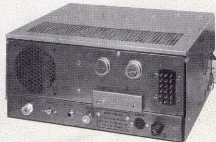
Rear panel input/output connections for accessories, antenna, key, ground, blower socket, fuseholder with fuse, power supply source.
