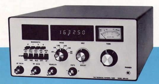
The GPR-110 is a highly sophisticated receiver with a basic range of 100 KHz to 30 MHz. It is solid state and stable to approximately one part in 10<sup>6</sup> without synthesis. A variety of options make it possible to accommodate the most exacting requirements of the user:
